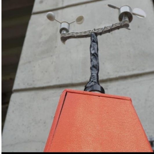
Image 8: Weather stations used on site by Adaptive Artifacts
